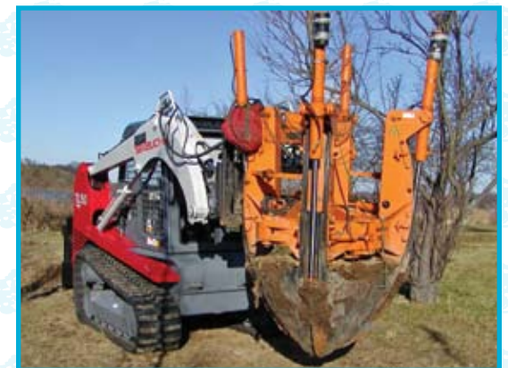
44" tree spade Moving up to 5" caliper
