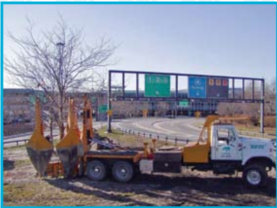
90" tree spade Moving up to 14" caliper
