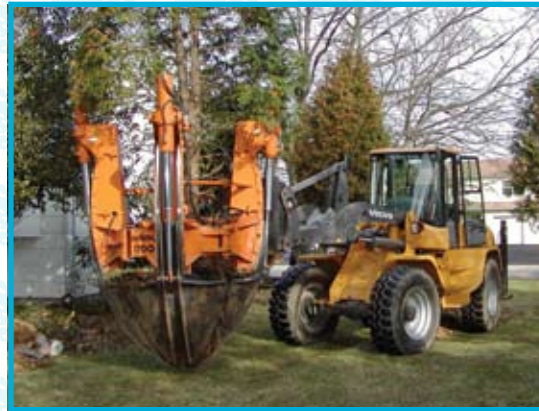
70" tree spade Moving up to 8" caliper
